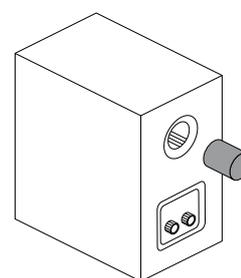
*To rightly match the sound of **Tesi 242** with the acoustics of your room, it is possible to change the bass frequencies level, simply fitting the supplied foam plug in the reflex vent: usually when the speaker is placed inside a recess.*
